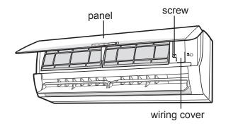
2. Make the power connection wire go through the cable-cross hole at the back of indoor unit and then pull it out from the front side.
