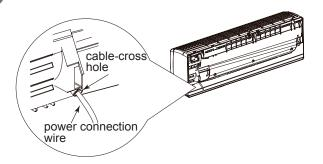
Remove the wire clip; connect the power connection wire to the wiring terminal according to the color; tighten the screw and then fix the power connection wire with wire clip.
